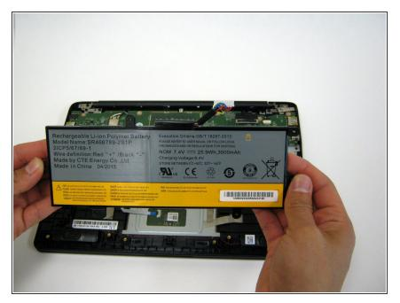
Lift the battery from the frame.
