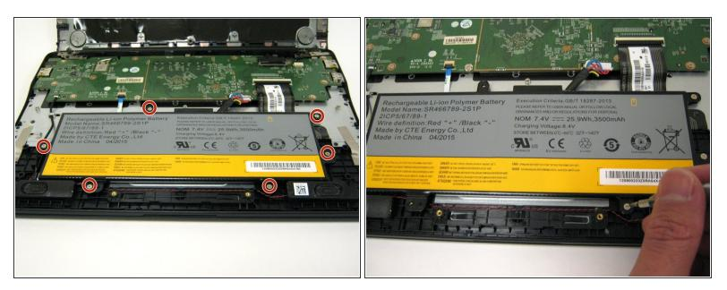
Remove the six 4mm screws using a Phillips #0 screwdriver.
