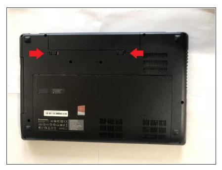
Slide out both locks for the battery, located on the back of the device.
