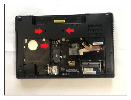
Unscrew the 3 "keyboard" detected screws.
