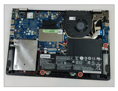
Remove the three 4 mm Phillips #0 screws holding the battery in place.
