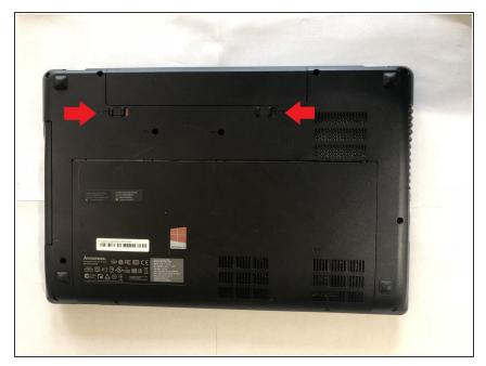
Slide out both locks for the battery, located on the back of the device.
