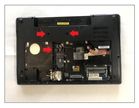
Unscrew the 3 "keyboard" detected screws.
