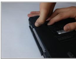
Slide and hold the two locking latches to the unlocked position.
