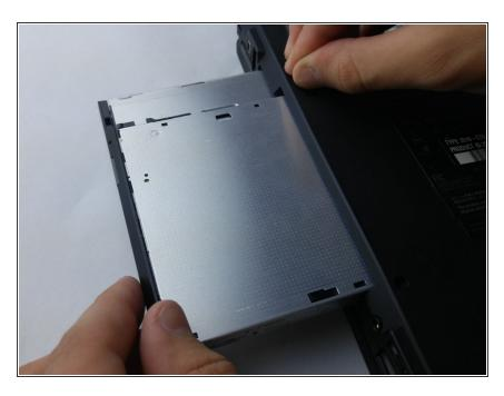
While holding the latches, slide the DVD drive away from the compartment and remove it from the device.
