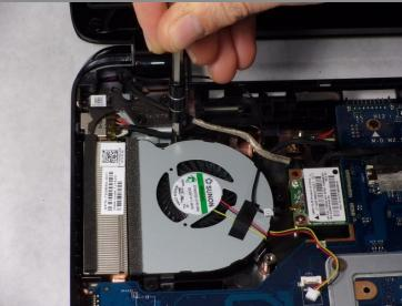
• Remove the three (3) 2.5mm by 3.5mm Phillips #0 screws from the fan.
