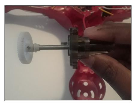
• Pull the gear out from the bottom of the holding mechanism.
