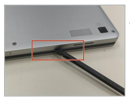
Using a plastic spudger, open the back cover and remove it from the laptop.
