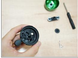
Use a spudger or a small metal bar to detach the end of the spring from the plastic that hangs off the circular base.
