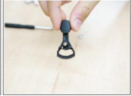
Put the components back to their original place in sequence, make sure the teeth of gears match.
