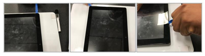
• With the back panel now removed, wedge the opening tools in between the actual tablet and screen and move it around parameter until you have loosened the adhesive keeping it together.
