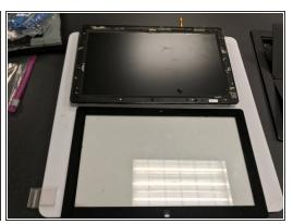
With your opening tool, remove the circuitry from off the main screen, thus separating the screen from the tablet completely
