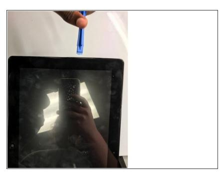
Wedge the opening tools inside the side of the device, and move it around the parameter until you have loosened the adhesive holding it together.
