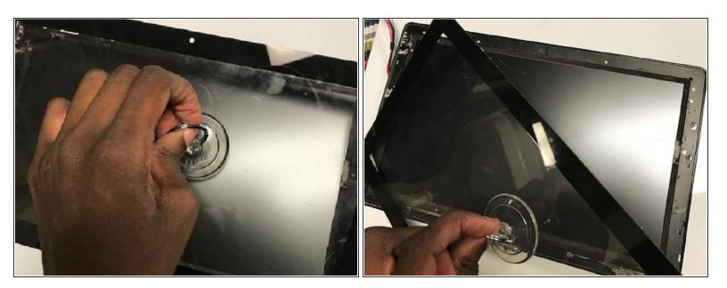
Place suction cup firmly on screen. When the cup is secure, lift up the screen and remove the screen.
