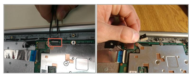
Remove the cable with tweezers as shown along the top of the board.
