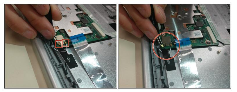
• Carefully pull off both brass connectors from the top left of the board with tweezers as shown.
