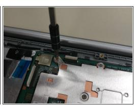
Remove the six screws from the board as shown. There are two types of screws here, so be careful to keep them separate for reassembly.
