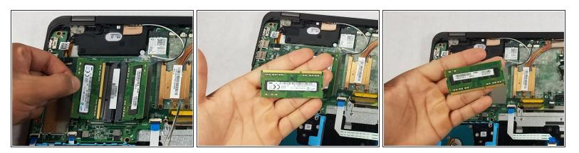
• Remove each RAM drive by pulling at an upwards angle in the direction of its free edge.
