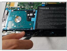
Remove the four 3mm Phillips #0 screws connecting the battery to the computer.
