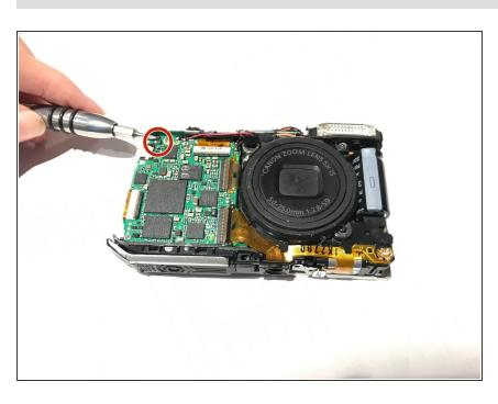
Using a JIS 000 screwdriver, remove the 1.2mm screw at the top left of the motherboard.
