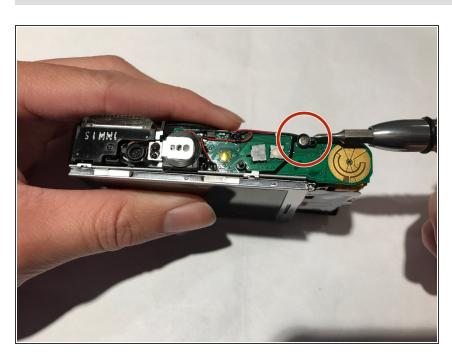
Remove the 1.6mm screw at the top of the camera.
