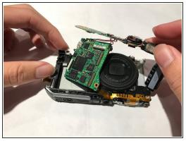
Remove motherboard and replace with a new one.
