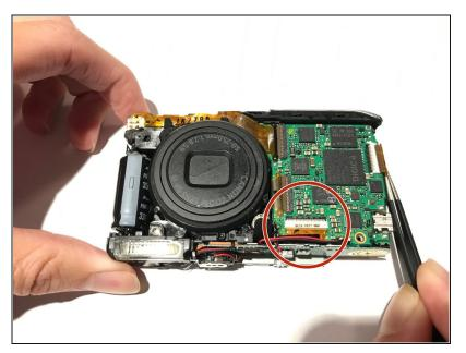
Use <u>tweezers</u> to pull out the circled brown flat flexible wire from its connection.
