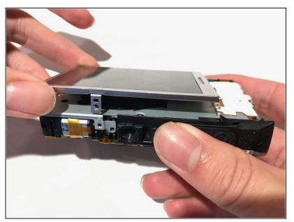
• Gently lift the LCD screen off the back of the camera.
