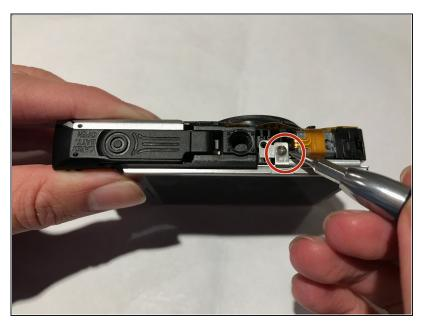
Use a JIS 000 screwdriver and remove the 3.0mm screw from the bottom housing.
