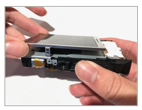
Gently lift the LCD screen off the back of the camera.
