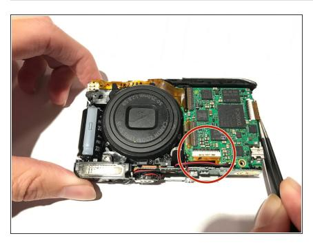
Use tweezers to pull out the circled brown flat flexible wire from its connection.
