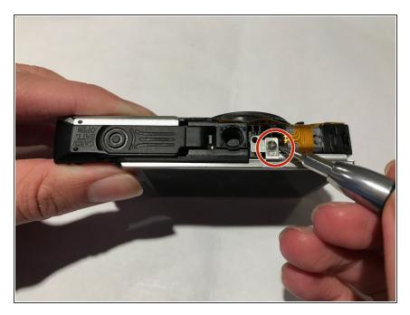
Use a JIS 000 screwdriver and remove the 3.0mm screw from the bottom housing.
