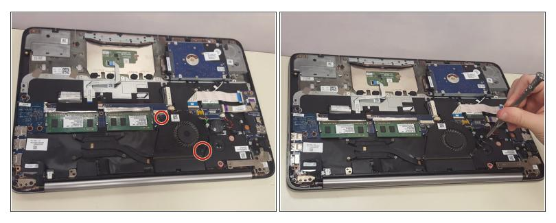
• Use the J0 screwdriver to remove the two M2.0x3.0 screws holding in the cooling fan
