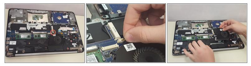
Unplug the cord and carefully remove the cooling fan
