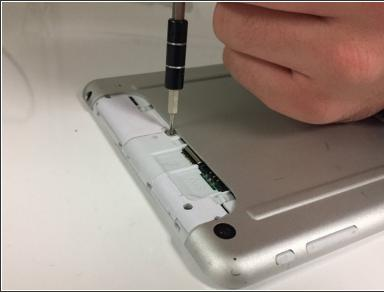
Using the Phillips Head #000, unscrew the 5 4mm and 3mm screws at the top.
