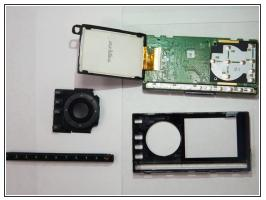
• Once the screws have been removed, the motherboard is free to come out.
