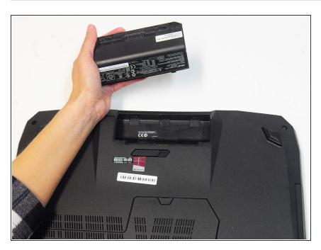
Remove the battery from its compartment.
