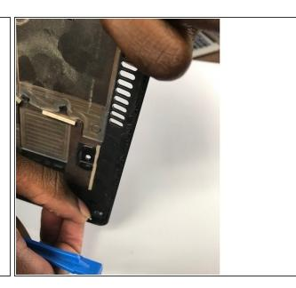
With the back panel already removed from the body of the tablet, push the power button(the button with the O/I symbol next to it) out of the panel from the inside. Do so with either your fingers or the removal tools.
