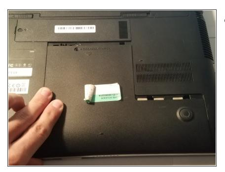
Using your hand slide the ODD/HDD/Memory panel off in a downward motion.
