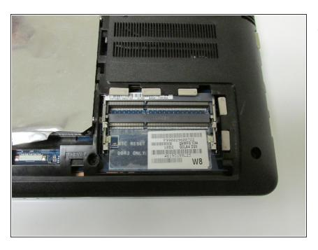
After removing all RAMs, the empty space looks like this. Then users can install the new RAMs.
