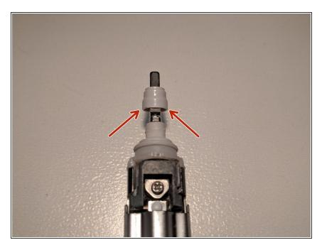
Use a puller to remove the plastic cap from the metal shaft to expose the defective rubber boot.
