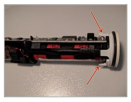
Remove the underside of the handpiece by carefully lifting the tabs at the two farthest vertexes of the oval with a small screwdriver.
