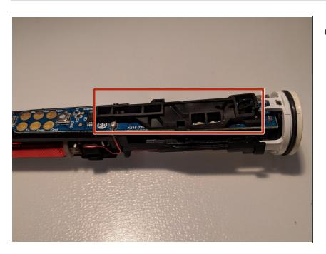
Remove the rubber pad from the motherboard
