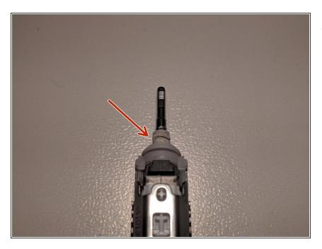
The defective rubber sleeve on the metal shaft must be replaced. A spare part is available for less than € 4 on eBay under the following designation: "Philips electric toothbrush Waterproof sealing parts for HX6730 HX6930 HX9340».
