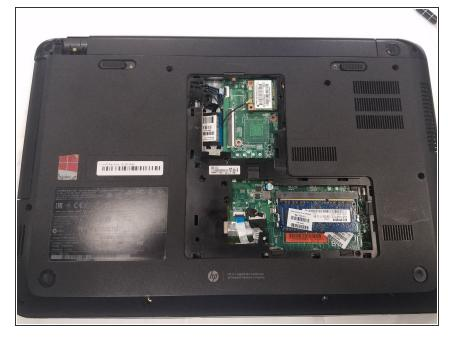
Once the back panel is completely removed you will have access to the RAM and many other connections in the computer.
