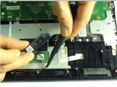
Detach the speaker cord from the hooks holding it to the frame and lift the speakers away.
