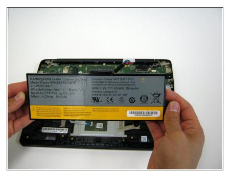
Lift the battery from the frame.
