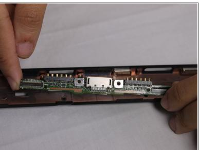
• The final step is to lift the keyboard port free from the frame using your fingers.
