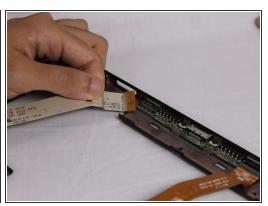
• Next, you need to remove the two ribbon cables located at the bottom of the frame. To detach the first ribbon cable you need to pull straight up on the orange connecter.
