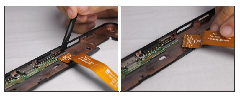
To remove the second ribbon cable you must first raise a black retainer with a thin plastic tool.
