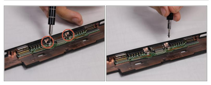
Now you must remove two 2.5mm screws that are securing the keyboard port to the frame. When removing the screws use the Phillips #000 bit.
