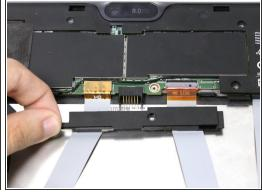
Slide the cover on the two middle ribbon cables out to remove it. It should uncover the orange cable connectors.
