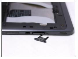
• Use your pin punch driver to push into the hole on the sim card, then pull out the sim tray.
