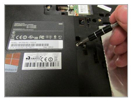
Locate and remove the M2.5X5 screw on the left hand side.
