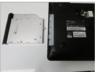
Pull out the CD drive and replace with the new one.
