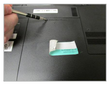
Using the Phillips #1 screwdriver, remove the M2.5X5 mm screw to take the back cover out.
