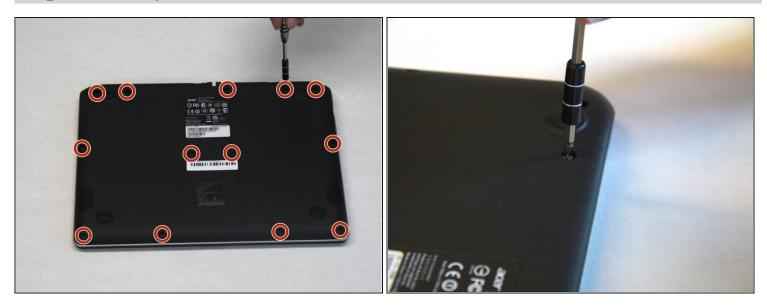
Remove the 13 indicated screws (6.2 mm) using a Phillips #1 screwdriver.
