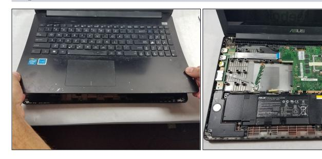
• Lift the keyboard assembly away from the remainder of the laptop.
