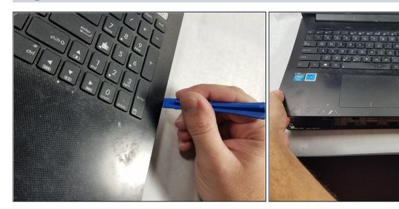
Use the Plastic Opening Tool to pry the keyboard assembly away from the rest of the laptop.
