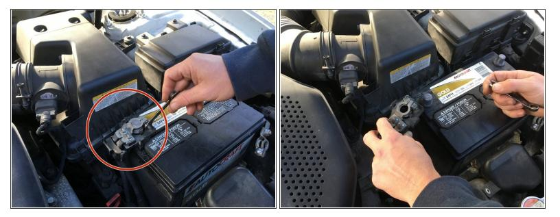
• Next, use the ratchet to loosen and remove (+) the positive cable.
