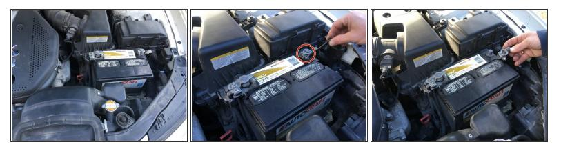
Locate the car battery and use the ratchet to loosen the negative (-) cable.
