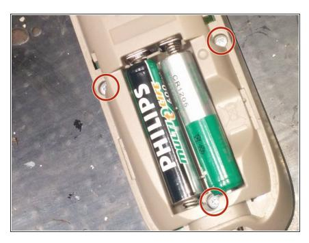
Remove the batteries and the 3 screws
