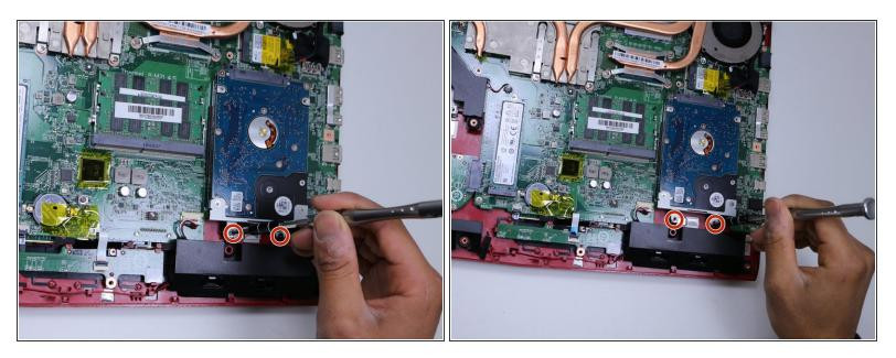
• Remove the two 5.5mm screws with the Phillips #1 screwdriver.
