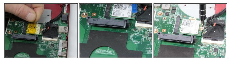
• Remove the WIFI card by disconnecting the two coax cables and removing the retaining screw.
