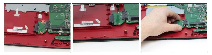
Use the Phillips #0 Screwdriver to remove the two 4mm screws that are holding the SATA connector in place.
