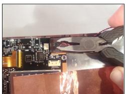
• Use small pliers to pull the connector, wiggling it a little as you pull it from its connection.
