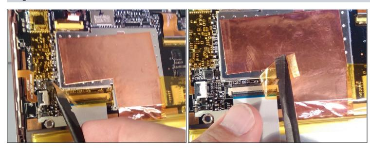
• Locate and remove the yellow cellophane tape from the display assembly ribbon cable ZIF connector.
