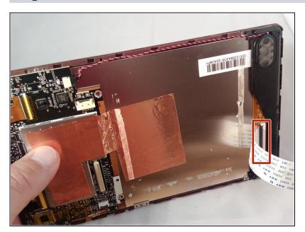
Locate the ZIF connector to remove the white ribbon cable
