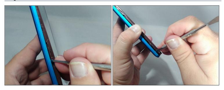
• Continue working the spudger downward and pry with the spudger until the bottom left-hand corner of the tablet is reached.
