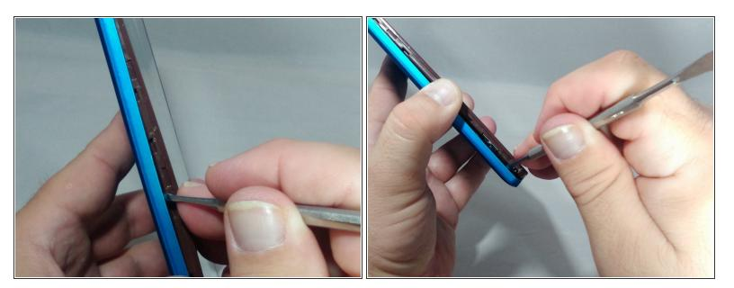
Continue working the spudger downward and pry with the spudger until the bottom left-hand corner of the tablet is reached.
