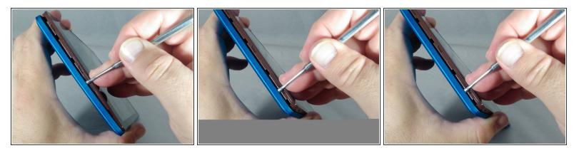
• Continue prying motion until the bottom right-hand corner of the tablet is reached.
