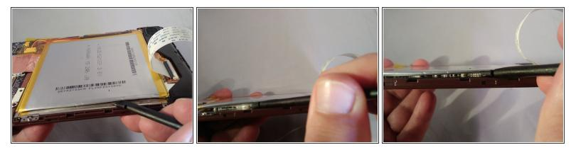
Move the spudger in a left-to-right scraping motion to loosen the glue until the battery is separated from the tablet.
