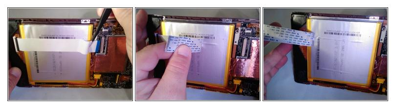
• Remove the white ribbon cable and carefully peel it off the battery.
