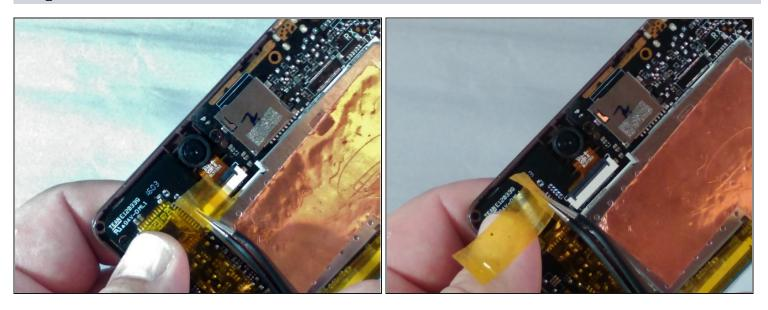
• Remove the yellow cellophane tape with the <u>tweezers</u> from the ZIF connector.
