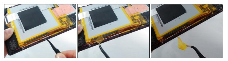
• Locate and carefully remove the yellow cellophane tape from the red and black speaker wires that connect the speaker to the edge of the motherboard.
