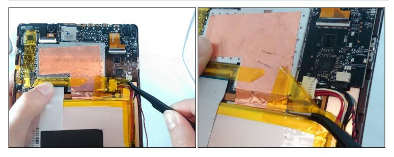
• Locate and carefully remove the yellow cellophane tape with <u>tweezers</u> from the battery connector and black and red speaker wires on the edge of the motherboard.
