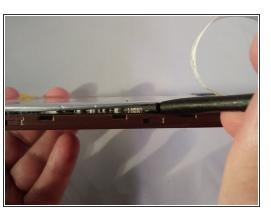
Move the spudger in a left-to-right scraping motion to loosen the glue until the battery is separated from the tablet.
