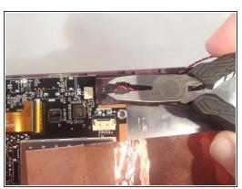
• Use small pliers to pull the connector, wiggling it a little as you pull it from its connection.
