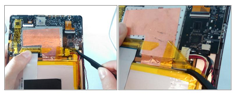
Locate and carefully remove the yellow cellophane tape with tweezers from the battery connector and black and red speaker wires on the edge of the motherboard.
