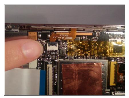
Locate the volume, power, home button ribbon cable ZIF connector.
