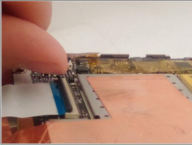
• Flip up the gray retainer clip on the white ribbon cable ZIF connector on the motherboard with your fingernail. If you do not have fingernails long enough, carefully use a black plastic spudger.
