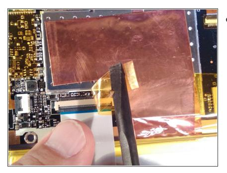
Locate the white ribbon cable Zero Insertion Force (ZIF) connector between the battery and the motherboard, and peel the yellow cellophane tape off the connector.
