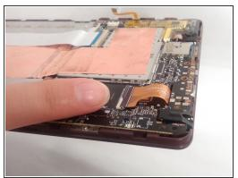
• Put your fingernail under the gray ZIF connector retainer and flip the retainer up. If you do not have fingernails long enough, carefully use a black plastic spudger.
