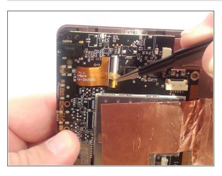
Locate the Display Assembly ribbon cable ZIF connector, and using tweezers, remove the yellow cellophane tape.
