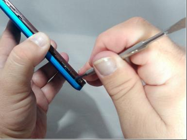
Continue working the spudger downward and pry with the spudger until the bottom left-hand corner
