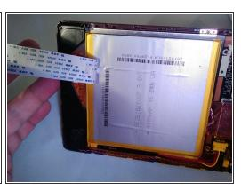
Remove the white ribbon cable and carefully peel it off the battery.
