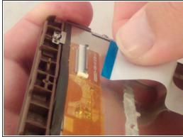
To remove the white ribbon cable, put your fingernail under the gray ZIF connector retainer and flip the retainer up.
