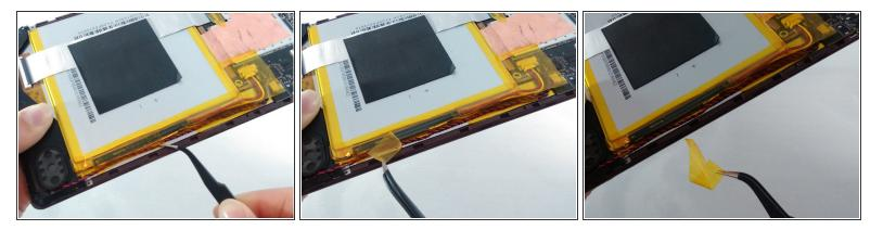
Locate and carefully remove the yellow cellophane tape from the red and black speaker wires that connect the speaker to the edge of the motherboard.
