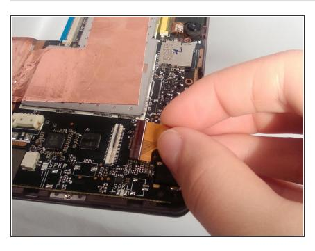
Remove the Display Assembly ribbon cable by gently pulling on it.
