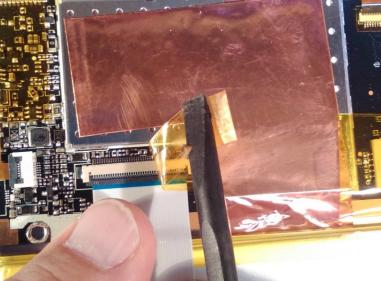
Locate and remove the yellow cellophane tape from the display assembly ribbon cable ZIF connector.
