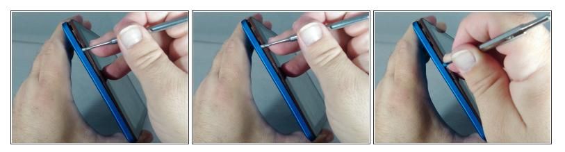
Along the bottom of the tablet, keep using a working and prying motion with the spudger to loosen the cover.
