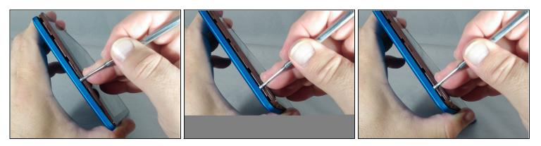
• Continue prying motion until the bottom right-hand corner of the tablet is reached.
