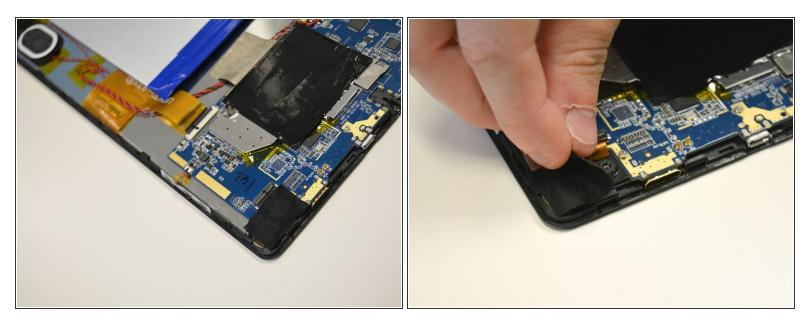
Once the back cover is removed, gently remove the black tape that covers the front and rear facing camera.
