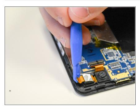
Near the edge of the device, lift up the tab connected to the front-facing camera.
