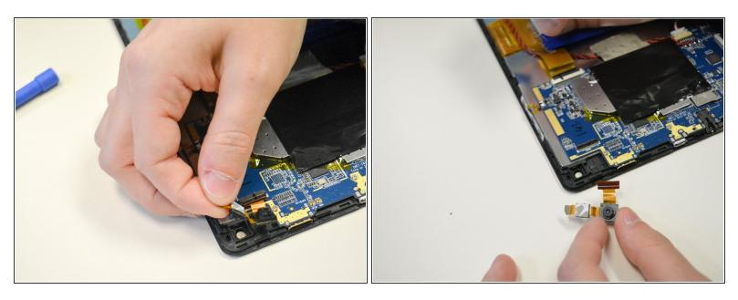
Gently pull on the tab connected to the front-facing camera to release both the front and rearfacing cameras.
