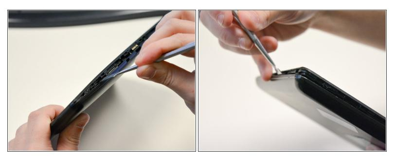
Continue to separate all of the clips around the device until the back cover comes off completely.
