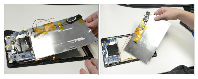
• Carefully slide out the metal slate and LCD screen from underneath the motherboard.
