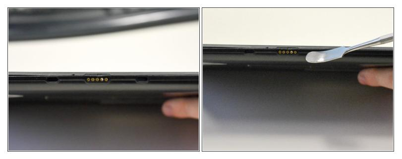
Locate the opening line between the cover and the device. Then locate the groove near the charging port.
