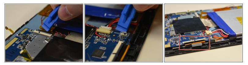
• Open the three black flaps located on each side of the motherboard.
