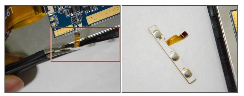
• Use the angled tweezers to pull the volume controls out and replace it with a new one.
