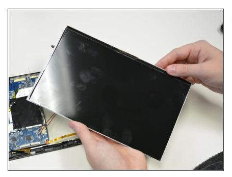
• Flip over the metal slate and separate the LCD screen from it.
