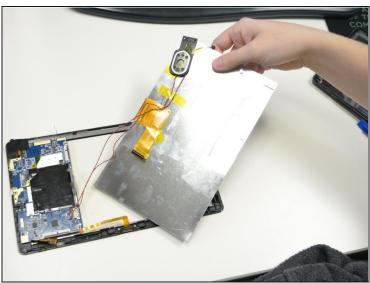
• Carefully slide out the metal slate and LCD screen from underneath the motherboard.
