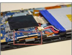
• Open the three black flaps located on each side of the motherboard.
