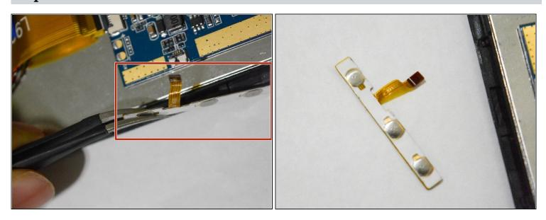
• Use the angled tweezers to pull the volume controls out and replace it with a new one.
