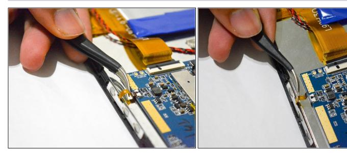
• Once the tab is released, use the angled <u>tweezers</u> to take out the tab.
