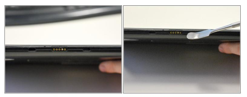
Locate the opening line between the cover and the device. Then locate the groove near the charging port.
