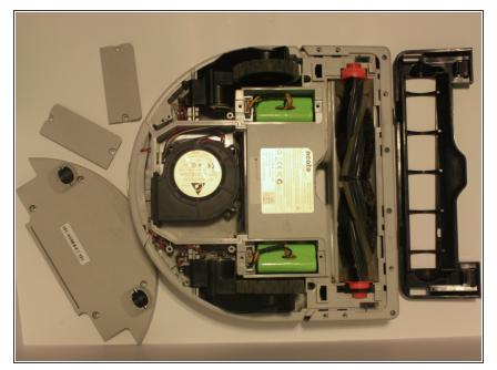
The Neato's core components are now exposed and ready to be cleaned and/or replaced.
