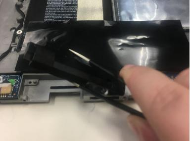
After unscrewing the speakers, gently lift the speaker out using the tweezers.
