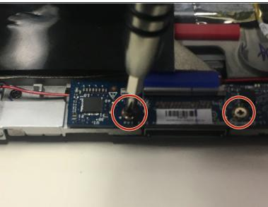
Once each speaker is out, remove the center plate in between the speakers, using the PH0 bit.
