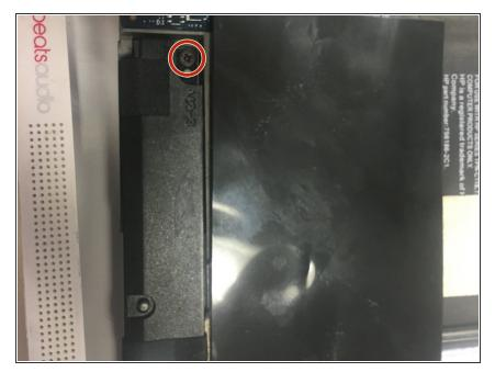
Using the PH 0 screw head unscrew each of the screws located int the upper right of the speakers.
