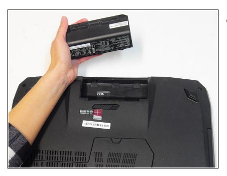
Remove the battery from its compartment.
