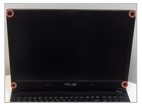
Remove the four 4mm Phillips #00 screws from the four corners of the display.
