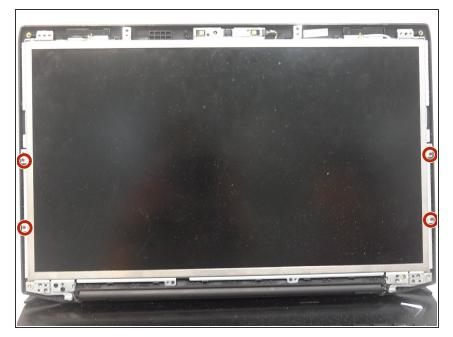
Remove the four 3mm Phillips #00 screws from the sides of the screen.
