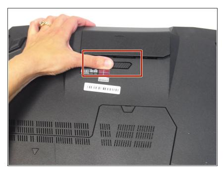
Slide the battery release latch all the way to the right. This will cause the battery to "pop" out slightly.
