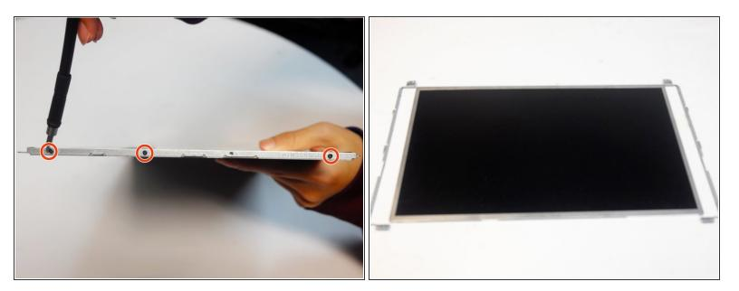
Remove the two side brackets from the sides of the screen by removing the six 3mm Phillips #00 screws attaching it. There are three screws on either side of the screen.
