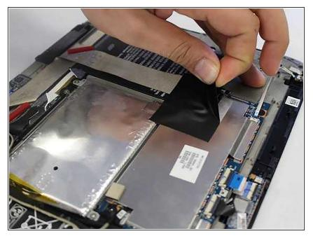
• Remove black stickers which is located on top of the battery.
