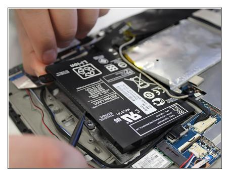
• Slowly lift up the battery as a whole and make sure the battery is remove on both ends.
