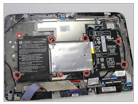
• Remove all eight 3mm Phillips screws using a J1 screw head.
