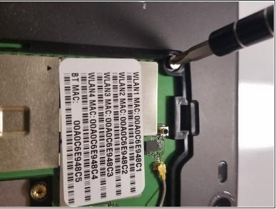
• Use the Phillips PH1 screwdriver to unscrew the five 4x2.5mm screws that hold the back cover.
