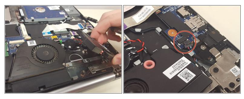
After unscrewing the screws, remove the speaker and carefully unplug it from the laptop.
