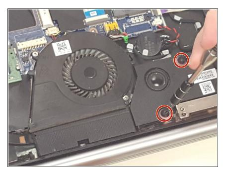
First, using a Phillips Head screwdriver, unscrew the two Phillips PM 2.5x5.5 screws that are connecting the speaker to the rest of the laptop.
