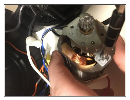
Use an electric screwdriver with a Phillips #1 head to take off the top metal piece.
