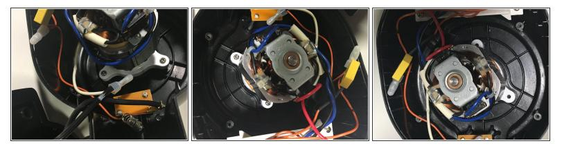
• Remove the three screws that hold the motor to the top case using a Phillips #1 screwdriver.
