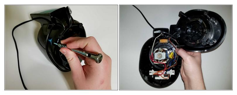
• Remove the back panel using a Phillips #1 Screwdriver on the four screws that hold it in place.
