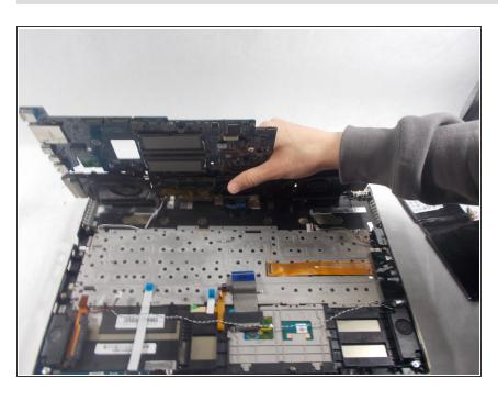
Lift the motherboard up and out of the device casing.
